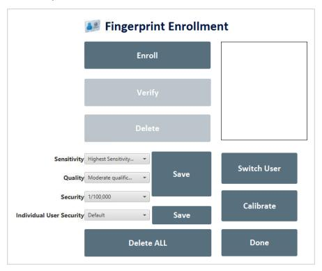
7. Instruct the employee to follow the on-screen instructions to capture the fingerprint, using the sensor on the top of the clock.
