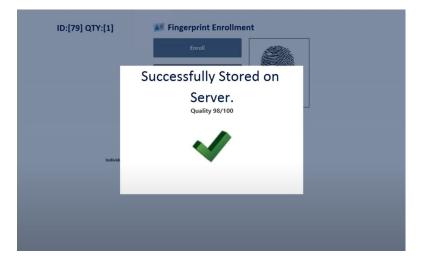
8. After successfully capturing the fingerprint, an image will appear, and the **QTY** in the upper left corner will change from 0 to 1.
